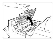
**2** Lift knob ① or knobs ① and ②, then remove any misfed paper.
